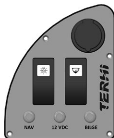
Figure 5. Terhi 450 CC control panel
